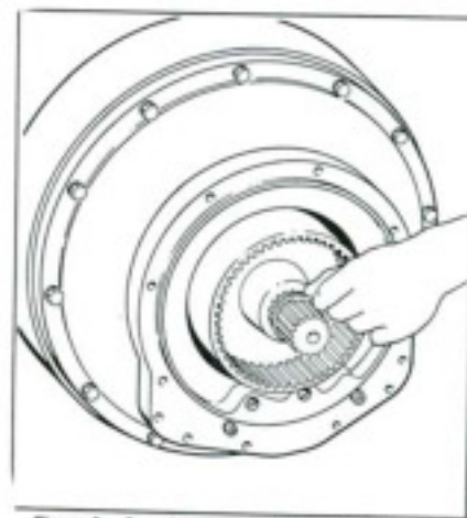
Figure 6. Securing Forward Clutch Driving Drum with Snap Ring.
